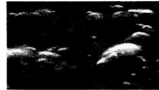
Electron micrograph, taken at 60° of nitrocellulose lacquer film containing Lo-Vel 27 flattening agent, 8% based on resin solids.
